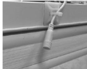
Internal Battery charging port
